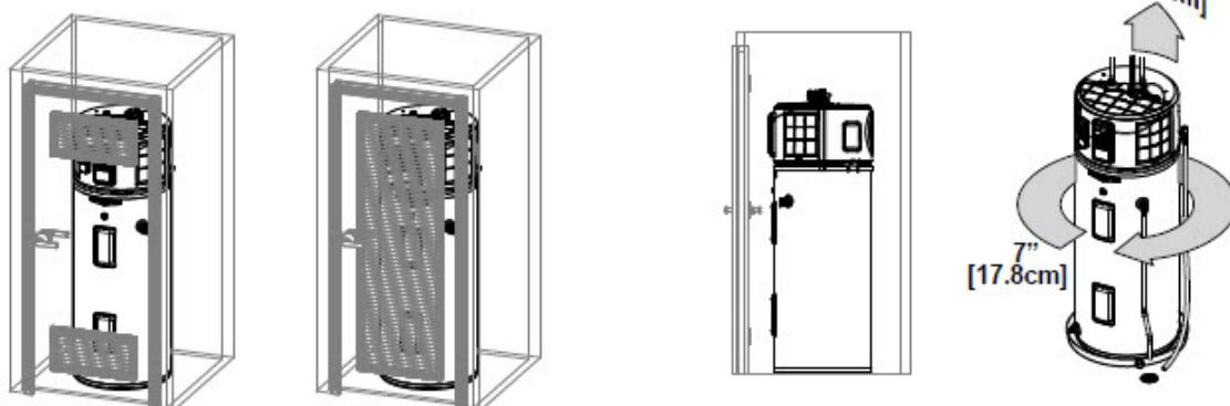
Enclosed closet space door should be fully louvered, or louvered at the top and bottom with a minimum of 300 in<sup>2</sup> open area. Top louvers should be above the units air intake.
