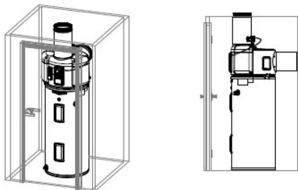
Door can be non louvered if closed closet space is ducted to an exterior air source.
